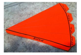
d. Score every line. Also score the curve. Bend at each place you have scored. Attach the tab to the lateral face farthest from it. Glue the bottom four tabs together.
